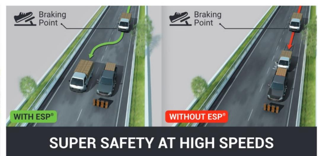
At highway speeds, ESP® gives better control during sudden braking, preventing instability.
