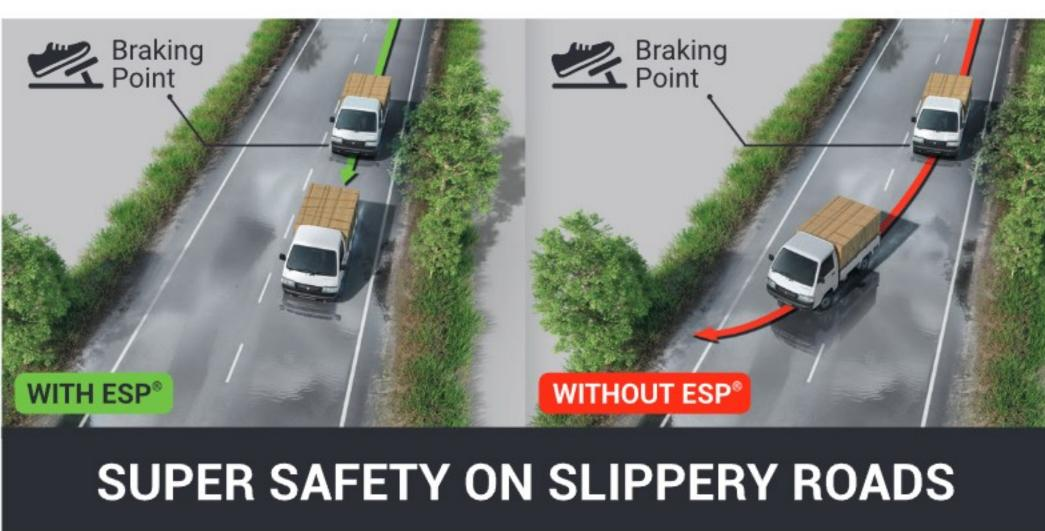
ESP® reduces skidding for better grip on wet surfaces, gravel, snow or loose soil.
